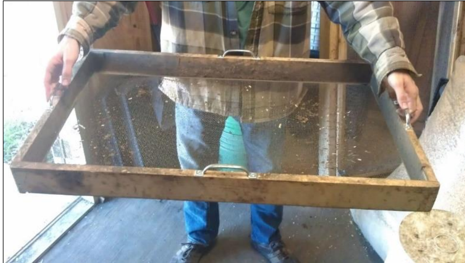
Figure 2. Hand screener used in screening vermicomposting castings in the study of an economic analysis of the development and management of a university vermicomposting system: a self-sustaining environmental and waste management educational tool.
