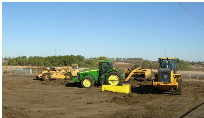
Figure 1. Manure harvesting equipment (from left to right: elevating scraper, tractor-pulled box scraper, and front-end loader).
