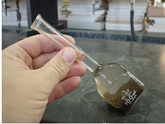
Figure 2. Agitating compost via swirling in a square based flask.
