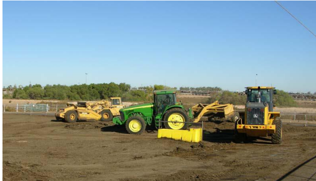
Figure 1. Manure harvesting equipment (from left to right: elevating scraper, tractor-pulled box scraper, and front-end loader). Source: Dr. Brent Auvermann, Texas AgriLife Research and Extension Center at Amarillo.
