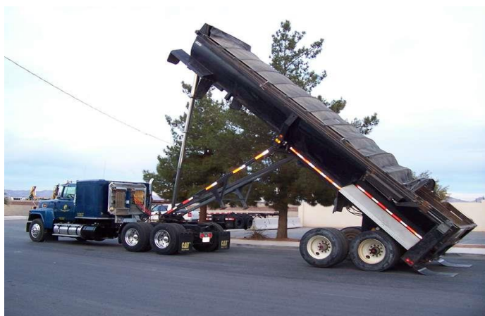
Figure 4. Manure harvesting equipment (End-dump tractor-trailer).
